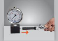
Press the thumb lever to disconnect coupler from the zerk fitting
